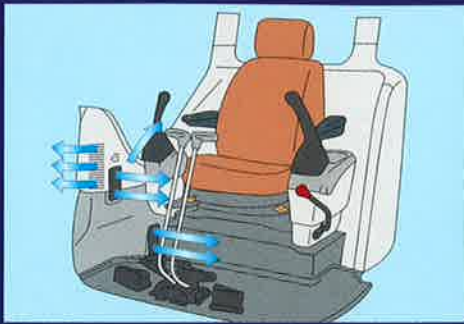
External flow, large-capacity air conditioner
